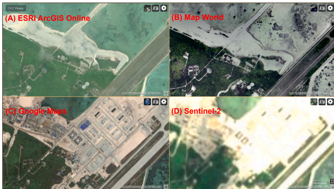
Fig. 4. Viewing local features when zooming in the imagery of the Woody Island. Each view shows the same locality, but the spatial resolution of the Sentinel-2 imagery (D) is evidently inferior to that of ESRI ArcGIS Online (A), Map World (B) or Google Maps (C).
