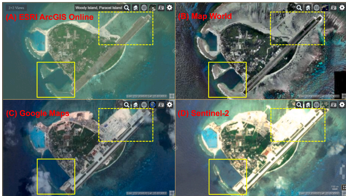
Fig. 3. Exploring the land reclamation project in the Woody Island, and comparing imagery layers released by several freely available imagery providers, including ESRI ArcGIS Online (A), Map World (B), Google Maps (C) and Sentinel-2 (D). All imageries show the same locality near the Woody Island. Yellow rectangles in the northeast and southwest of the island indicate the locations with significant differences caused by the reclamation project. (For interpretation of the references to colour in this figure legend, the reader is referred to the web version of this article.)
